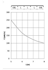
Cable ladder for large support distances up to 8 metres Perforated C datarungs 41x21 With floor plate
